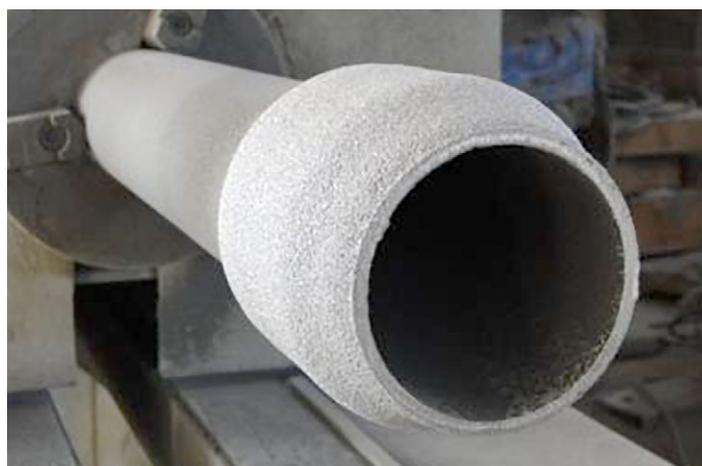
A thick coating of Metco 8280 hand-sprayed at a distance of 200 mm (8 in). Notice the light gray, metallic appearance of the coating.
